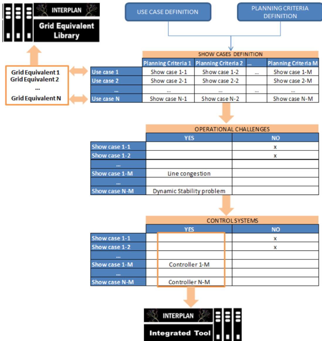
Figure 3: Relationships between operation planning inputs and INTERPLAN tool components
